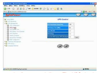
shutdown delay time set in the Shutdown Program in all connected clients. The UPS shutdown delay time set in WebPower should always be greater than the shutdown delay time set in the Shutdown Program
