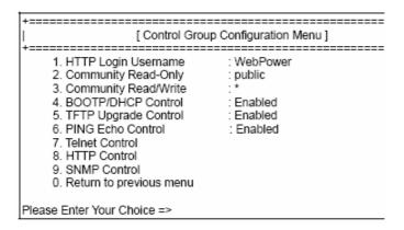
Attention: If your Network environment is static IP address, please set DHCP as disabled and then restart WebPower. Connect RJ-45 cable when WebPower started.
